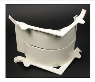
Radiused insert for 4017 Internal Elbow and 4018 External Elbow in divided or undivided applications. Provides 2" (51mm) cable bend radius control for UTP, STP and fiber optic cable installations. Ideal for new and retrofit applications whether the cable installation is layin or pull-through.
