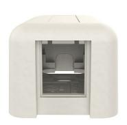
HDJ Surface Mount Boxes accept rear loading High Density jacks & modules and provide easy snap-on covers and snap-in label fields. Boxes are supplied with screws and double-sided adhesive tape for mounting onto almost any surface. Meet UL2043 and are suitable for installation in air handling spaces (ie plenum spaces).
