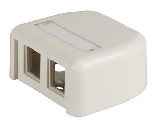
HDJ Surface Mount Outlet Boxes accept rear loading High density Jacks & modules and provides easy snap-on covers and snap-in label fields. Boxes are supplied with screws and double-sided adhesive tape for mounting onto almost any surface. Meet UL2043 and are suitable for installation in air handling spaces (ie plenum spaces)
