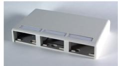
Ortronics Series II Surface Mount Outlet Boxes accept front-loading Series II modules and provide snap-on covers and snap-in label fields. Boxes are supplied with screws and double-sided adhesive tape for mounting onto almost any surface. Compatible with Wiremold 2700, 2800 and 2900 raceway series.
