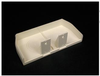
Closes off raceway end runs. Can be used to feed raceway using 1/2" or 3/4" trade size conduit. Holes for conduit must be drilled. Use a step drill or other means.
