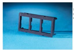
This plate accepts three TracJack modules or blanks. Use with 40700071, 40700072, or 40700073 bezels, to snap mount into 2.70'' x 1.375'' TIA referenced furniture openings for Steelcase, Haworth, Knoll and others. 5 pack.
