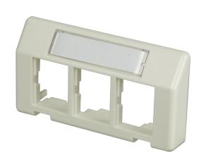
This plate has 3 Front-load jack openings for Tracjack (TJ) modules or blanks, snap mounts into 2.70" x 1.375" TIA referenced furniture openings for Steelcase, Haworth, Knoll and others.
