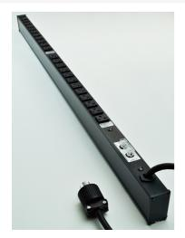
Two circuits with two 20A resettable circuit breakers. Twenty-four 20A outlets with T-slots, black housing. 12' (3.6m) cord. Length 48'' (1.3m).
