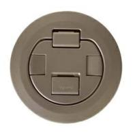
Surface style die-cast aluminum cover assembly with powder coated finish. 4CTC Series cover assemblies designed for use with 4STC Poke-Thru Stem Assemblies . NOTE: Add suffix "TR" to the end of the part number to indicate tamper-resistant cover assembly.
