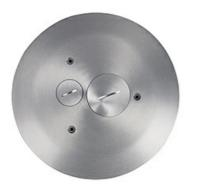
Complete with one 3/4" and one 1 1/2" trade size conduit adapters and closure plugs. Covevrs available in painted black (BK), gray (GY), brass(BS), nickel (NK), bronze (BZ), and forged brushed aluminum (AL). Use with the 4FFSTC15 insert to form a complete poke-thru assembly. NOTE: Assembled with scrub water gasket. For use on tile or carpet floors. 4FFATC Series Poke-Thru Devices require a 4" (102mm) diameter hole.
