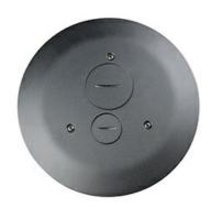
Complete with one 3/4" and one 1 1/2" trade size conduit adapters and closure plugs. Covevrs available in painted black (BK), gray (GY), brass(BS), nickel (NK), bronze (BZ), and forged brushed aluminum (AL). Use with the 4FFSTC15 insert to form a complete poke-thru assembly. NOTE: Assembled with scrub water gasket. For use on tile or carpet floors. 4FFATC Series Poke-Thru Devices require a 4" (102mm) diameter hole.
