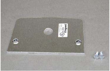
Single receptacle faceplate. Hole diameter: 7/8" (22.2mm). NOTE: Four-piece service fittings include: housing and base plate. Receptacles included when indicated in part number description. 525 Series Service Fittings have 27 cubic inches (442ml) of capacity.
