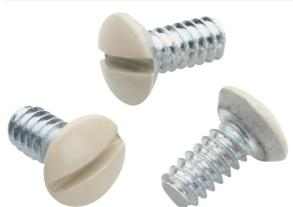
Oval head milled slot. • 1/2" long, 6x32 thread. • Standard size for duplex receptacles and toggle switch wall plates. • Ivory.
