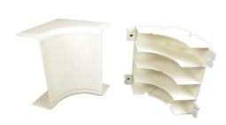
For right angle turns around internal corners. Integral dividers provide 2" (51mm) cable bend radius for UTP and Fiber Optic installations. Ideal for lay-in or pull-through installations.
