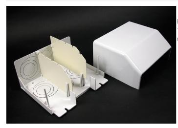
For feeding raceway from larger conduits. Has concentric 3/4", 1", 1 1/2", and 2" trade size KOs on end and back. Two removable dividers are included.
