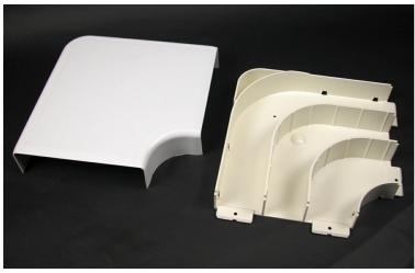
90 degree flat corner, with integral dividers, that provides a 2'' (51mm) cable bend radius for UTP and fiber optic installations. Ideal for lay-in or pull-through installations.
