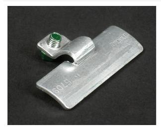
Provides additional grounding for 500 or 700 Series Raceway or to ground remotely HICated devices. Insert clamp into raceway before installing. Attach ground wire to screw as required by National Electrical Code.
