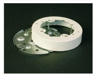
Cover accepts fan bracket device with mounting centers of 3 3/16" [81mm]. Base has six mounting holes and 4 1/2" trade size KOs. #10 mounting studs provided. Rated for fans and fixtures up to 50 lbs. NOTE: Certified to Canadian Safety Standards for sale in Canada. When ordering these products, change the "V" color prefix to "vc" or the "WH" color suffix to "WHC" to denote the Canadian versions.
