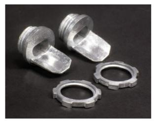
Male conduit connector with 1/2inch trade size conduit opening for connecting Wiremold 500/700 Series raceway to conduit boxes or panel boxes that have KOs for conduit. Can also be used with conduit type fittings. When used with 700 Series Raceway, break out crescent twistout in connector.
