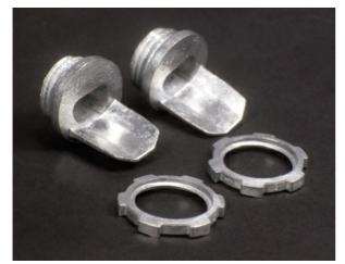
Male connector with 3/4" trade size conduit opening for connecting raceway to conduit boxes or panel boxes that have KOs for conduit. Can also be used with conduit type fittings. When used with 700 Series Raceway, break out crescent twistout in connector.
