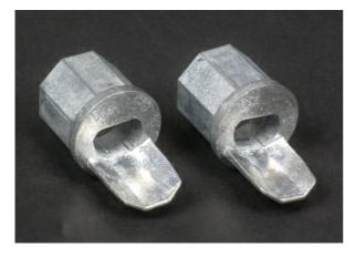
Interior threaded female connector with a 3/4" trade size conduit opening for connecting raceway to conduit. When used with 700 Series Raceway, break out crescent twistout in connector.
