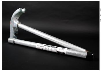
For making smooth, accurate bends, saddles and offsets in Wiremold 500 and 700 Series Raceways. Two0piece handle fits in tool box.
