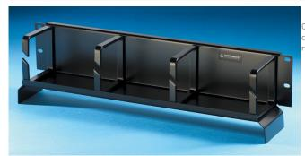
Ortronics bend limiting cable management panels have curved falls that protect against cable crimping and also maintain proper bend radius. The panels are ideal at the top of standard 19" EIA racks. 3.5"H x 3.5"D rings with waterfall, 2 rack units, black.
