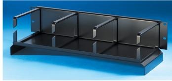
Ortronics bend limiting cable management panels have curved falls that protect against cable crimping and also maintain proper bend radius. The panels are ideal at the top of standard 19" EIA racks. 3.5" H x 6" D rings with waterfall, 4.84" H x 19" W, 2 rack units, black.
