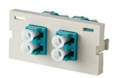
The Series II, Dual, Multimode, LC Duplex, Aqua Adapters (4-Fiber), Beige Adapter Plate, has two duplex adapters with 180 Degree exit, and ceramic alignment sleeves. This adapter panel is 1 unit high. These adapter panels include dust caps, and offers two insests for optional icons (Not Included), to label each connector and indicate its purpose. Compatible With: Series-II Workstation Face Plates and Series-II Workstation Surface Mount Boxes. Wiremold raceway series 2700, 2800, and 2900
