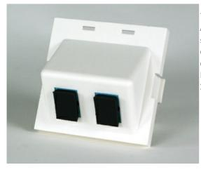
The Series II, Dual, Multimode, SC Simplex, Aqua Adapters (2-Fiber), White Adapter Plate, has two simplex adapters with 180° exit, and ceramic alignment sleeves. This adapter panel is 2 units high. These adapter panels include dust caps, and offers two insests for optional icons (Not Included), to label each connector and indicate its purpose. Compatible With: Series-II Workstation Face Plates and Series-II Workstation Surface Mount Boxes. Wiremold raceway series 2700, 2800, and 2900
