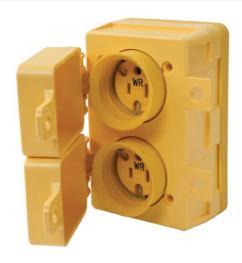
Straight Blade Watertight Duplex Receptacle, 15amp 125volt, NEMA Configuration 5-15R, Impact resistant Valox lid, cover plate, and receptacle body withstand impacts, chemical, and corrosion.
