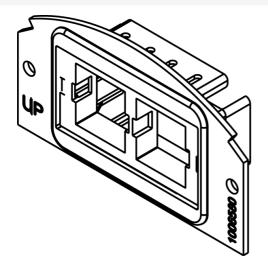
Device plate that will accept up to two (2) ports of communication devices. For use in either of the two side compartments only. Not for use in the center compartment. Communication devices supplied by others.
