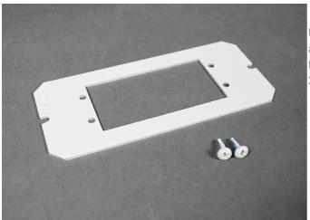
Used for floor coverings greater than 5/16" (7.9mm). The 6TS will allow the top surface of the cover to be flush with the finished floor. Includes six (6) 1/16" (1.6mm) thick shims. Up to a total of 3/8" (9.5mm) of adjustment.
