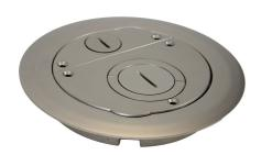
Surface style, die-cast aluminum cover assembly with one (1) 3/4inch trade size screw plug opening, and one (1) concentric 2inch -1 1/4inch trade size screw plug opening. Cover assembly is available in the following powder coated finishes: (BK) black, (GY) gray, (NK) nickel, (BS) brass, and (BZ) bronze. 6CFFTC Series cover assemblies designed for use with 6STC Poke-Thru Stem Assemby. Includes one (1) 3/4inch and one (1) 1/2inch trade size conduit fittings and one (1) divider to separate devices.
