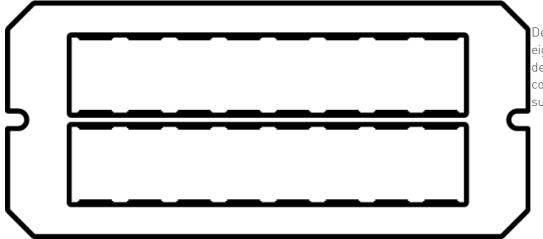
Device plate that will accept up eight (8) Ortronics TracJack devices. For use in the center compartment only. Devices supplied by others.
