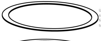
Used for floor coverings greater than 5/16" (7.9mm). This tile shim will allow the top surface of the cover to be flush with the finished floor. Includes six (6) 1/16" (1.6mm) thick shims. Up to a total of 3/8" (9.5mm) of adjustment.
