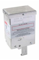
Three pole, Three Phase AC Manual Motor Controller 30 amp, 600 watts., Suitable as Motor Disconnect - 10KA @ 600VAC, 30A max Class J fuse.
