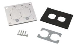
Brushed aluminum duplex cover plate, for OmniBox® and Modulink<sup>™</sup> Series floor boxes. Cover plate is 3.290 inch x 4.310 inch (83.6mm x 109.5mm). Flip lids can also be used with 106 type frames for communications. NOTE: Brass covers and flanges are not interchangeable with aluminum or nonmetallic covers and flanges. Nonmetallic covers are interchangeable with aluminum flanges.
