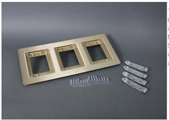
Three gang brass combination carpet and tile flange, for OmniBox® and Modulink™ Series floor boxes. Flange is 6.080 inch x13.310 inch (154.4mm x 338.1mm). Accepts Ortronics MAB6TJ TracJack and MAB3S2 Series II, and Wiremold CM Series Open System adapters, sold separately. NOTE: Brass cover plates can only be used with brass flanges. Brushed aluminum flanges come with beveled edges.
