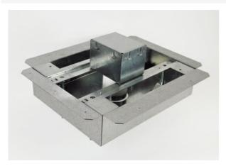
1-Gang Fire Classified Steel Floor Box. Adjustment range over deck of 2" (51mm) minimum to 5" (127mm) maximum. Use in normal weight concrete 4 1/2" (114mm) minimum pour over deck. One 1 1/4" (32mm) conduit feed opening. Box Capacity 53 cubic inches. This floor box preserves the 2-hour fire rating of floors in which it has been installed.
