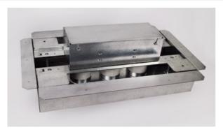
3-Gang Fire Classified Steel Floor Box. Adjustment range over deck of 2" (51mm) minimum to 5" (127mm) maximum. Three 1 1/4" (32mm) conduit feed openings. Inside Gang Capacity - 67.5 cubic inches. Outside Gang Capacity - 54 cubic inches each gang. This floor box preserves the 2-hour fire rating of floors in which it has been installed.
