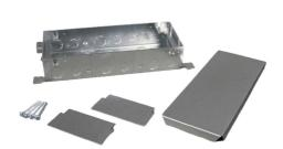
The 880M3 shallow three gang Omnibox® Floor Box provides an excellent activation solution for applications where multiple services are required in open space areas. The 880M3 floor box is offered in a stamped steel construction, designed to be installed in above grade concrete floor applications and to meet a wide range of market requirements.
