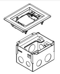
880W1 Floor Box with 817B Brass Flange included. Flange can be used for tile or carpet applications. Order cover separately.
