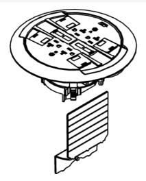
For 881PVC Floor Box. Kit complete with two (2) 20A duplex receptacles, (receptacles can be wired as standard or Isolated Ground), flange and slide holder, 881ADP Adapter, and 881DIV Divider. Provided with Wiremold CM Series Open System unloaded adapters, Ortronics Series II and TracJack adapters. Modular jacks sold separately. CAUTION: Not for use on concrete pours less than 4 1/2'' (114mm) deep. Not for use when concrete is the finished floor. Use only for tile, carpet, or wood covered floors.
