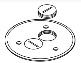
Brass cover plate with two screw plug openings, 5 1/2" (140mm) for carpet. NOTE: For carpet or tile installations. All cover plates are furnished with gasket and three screws. The 895P Polycarbonate Series Cover Plates must be field modified for dual service.
