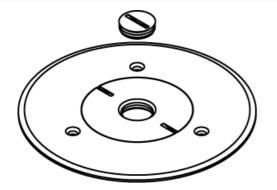
Brushed aluminum (896CKAL-1/2) cover plate with 1/2" (12.7mm) threaded opening 5 1/2" (140mm) for carpet. NOTE: For carpet or tile installations. All cover plates are furnished with gasket and three screws. The 895P Polycarbonate Series Cover Plates must be field modified for dual service.
