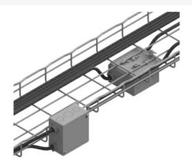
This junction box can be directly installed on the side, bottom or corner of any CF series Cablofil wire mesh tray. Unique design allows secure attachment with a 45° twist. Available in two sizes, TC4 and TC5 junction box assemblies feature quality construction and bonding holes for quick and secure attachment.
