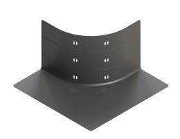
Radius shields create a smooth corner around junctions made with EZT90 and RADT90 hardware. They're made from durable, black ABS plastic and include slots for mounting with zip ties. Radius shield is available in one size - just trim to fit your installation tray depth.
