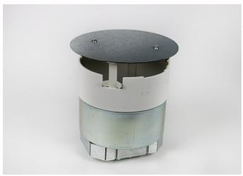
Complete abandonment plug assembly for 6" opening. Assembly includes intumescent fire stop material to maintain a 2 hour fire rating of the floor.
