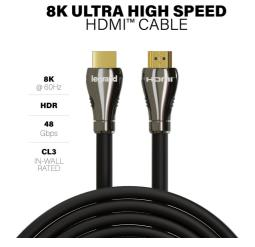
This Ultra High-Speed (48Gbps) HDMI cable supports 8K at 60Hz and 4K at 120Hz. It is CL3/FT4 rated for in-wall use and includes a Sure Grip connector for a firm hold to prevent cable damage. Enhanced retention clips ensure the cable stays securely in place, and the gold-plated connector provides excellent corrosion resistance and signal conductivity. The Enhanced Audio Return Channel (eARC) supports high-bitrate audio formats such as DTS-HD Master Audio, DTS:X, Dolby TrueHD, and Dolby Atmos.
