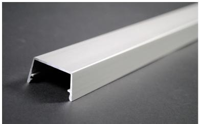
1 7/16" (37mm) wide, 6063-T5 extruded aluminum, satin anodized finish, .60" (1.5mm) nominal thickness. Cover packed (12) 5' (1.5m) lengths per carton.
