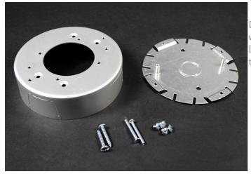
Designed for use in hanging fixtures. Cover takes any device with mounting screw centers of 2 3/4", 3 1/2" and 4 1/16" (70mm, 89mm, 103mm). Base has concentric 1/2" and 3/4" trade size Kos.
