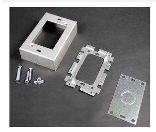
Single Gang Shallow Device Box. Designed for standard shallow switches and receptacles. Base has open back plate for mounting to existing wall box and solid black plate insert with 1/2" and 3/4" trade size Kos to close opening.
