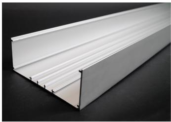
6063-T5 extruded aluminum, satin anodized finish, .080'' (2.03mm) wall thickness. Base has four ribs for snap-in divider. This base is packed eight 5' (1.5m) lengths per carton.
